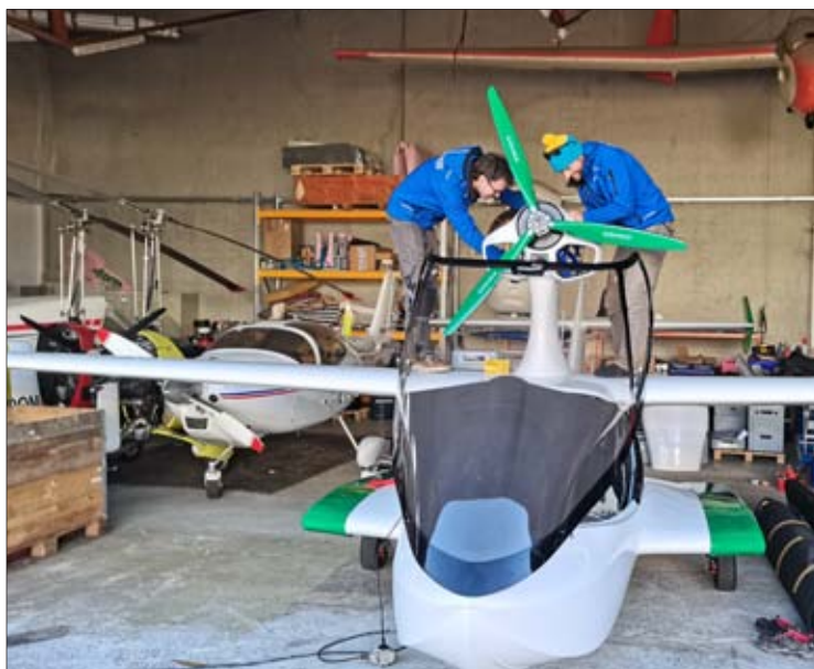
Installation work on the electric drive unit 检查 DS 2C 的电驱
