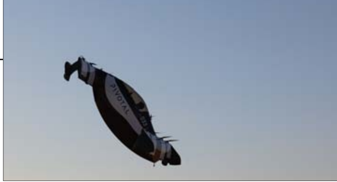
Tilt aircraft: During takeoff, the aircraft rotates around the pilot into a vertical flight position. Helix 是尾座式 eVTOL：起飞时，飞机围绕飞行员旋转过渡到垂直飞行姿态。
