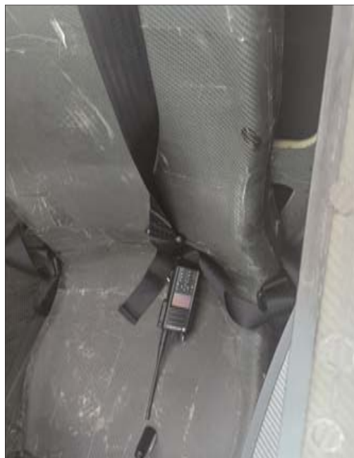
Fast charging: The 8 kWh battery can be charged simultaneously via two charging ports (left). A ballistic rescue system is also installed (bottom left). All software was developed in-house (bottom). Spartan seating: For reasons of weight, a carbon seat shell has to suffice in an ultra-light aircraft (right).
