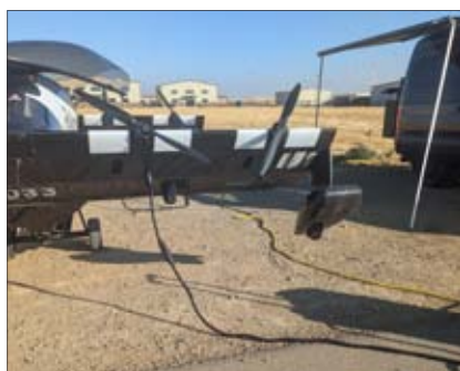
Fast charging: The 8 kWh battery can be charged simultaneously via two charging ports (left). A ballistic rescue system is also installed (bottom left). All software was developed in-house (bottom). Spartan seating: For reasons of weight, a carbon seat shell has to suffice in an ultra-light aircraft (right).
