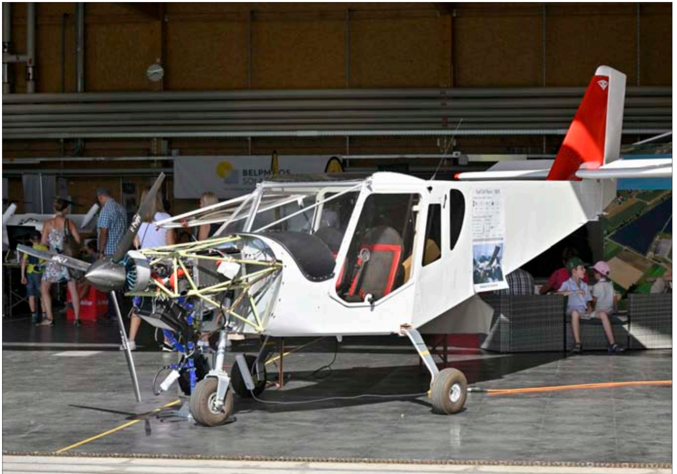
IBMS converted this Zenair CH 750 into an electric aircraft. The power supply is provided by a combustion engine. The electric motor has an output of 75 kW.
